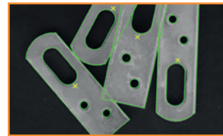
Industry-proven shape-based matching for robust localization of objects
