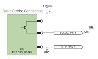
\*External resistors may not be needed Check documentation on I/O for recommendations and voltage limits
