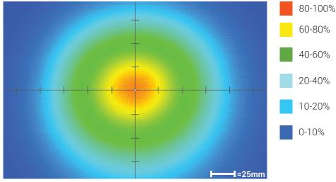
Optical measurement taken using SL-S050075M-WHI @ 300 mm
