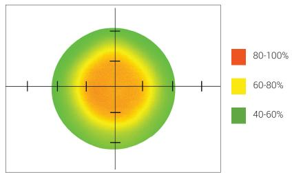
Optical measurement taken using RL1660-66035I3 @ 25 mm
