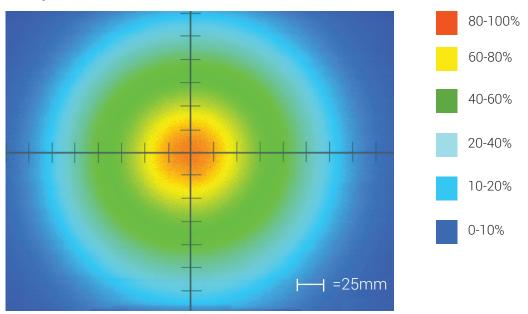
Optical measurement taken using RL-S052120M-WHI @ 300 mm
