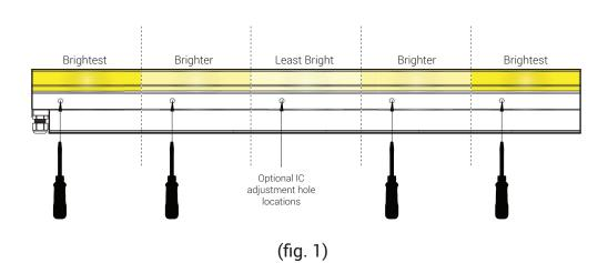
Controlling each 6" (152mm) section independently and making the center of the line less bright and
