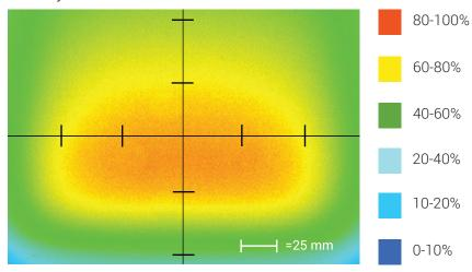
Optical measurement taken using DL085-WHI24 @ 25 mm
